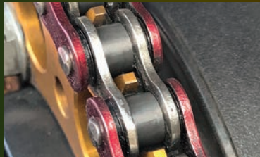
well-lubricated and in good condition
