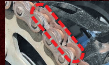
insufficient lubrication, roller wear
