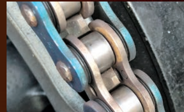
dry surface, lack of lubrication
